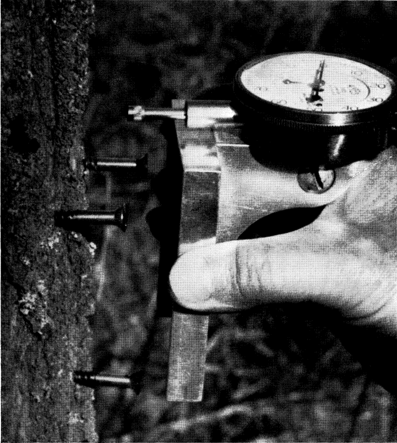
Dendrometer made by attaching a machinist's dial gauge to an aluminium platform which is placed against permanently set screws. A rim around the sides and top of the platform allows exact replacement of the instrument if the rim is fitted against the top two screws in the same manner at sequential readings. The screws penetrate the tree for more than half their length. (Photograph by R. Daubenmire.)
